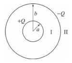
90. Two thin, concentric, spherical conducting shells are arranged as shown in the figure above. The inner shell has radius a, charge +Q, and is at zero electric potential. The outer shell has radius b and charge -Q. If r is the radial distance from the center of the spheres, what is the electric potential in region I (a < r < b) and in region II (r > b)?
