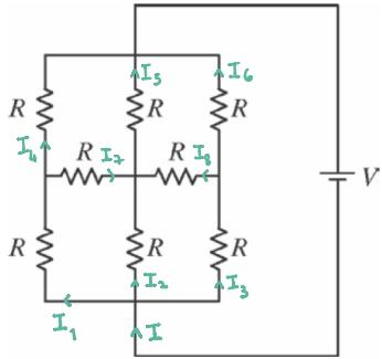
68. The circuit shown in the figure above consists of eight resistors, each with resistance  $R$ , and a battery with terminal voltage  $V$  and negligible internal resistance. What is the current flowing through the battery?
