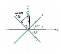
60. Three long, straight wires in the xz-plane, each carrying current I, cross at the origin of coordinates, as shown in the figure above. Let  $\hat{\mathbf{x}}$ ,  $\hat{\mathbf{y}}$ , and  $\hat{\mathbf{z}}$  denote the unit vectors in the x-, y-, and z-directions, respectively. The magnetic field  $\mathbf{B}$  as a function of x, with y = 0 and z = 0, is
